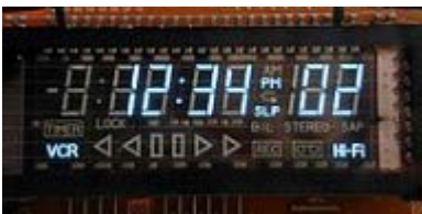
Figure 8 — Vacuum Fluorescent Display
